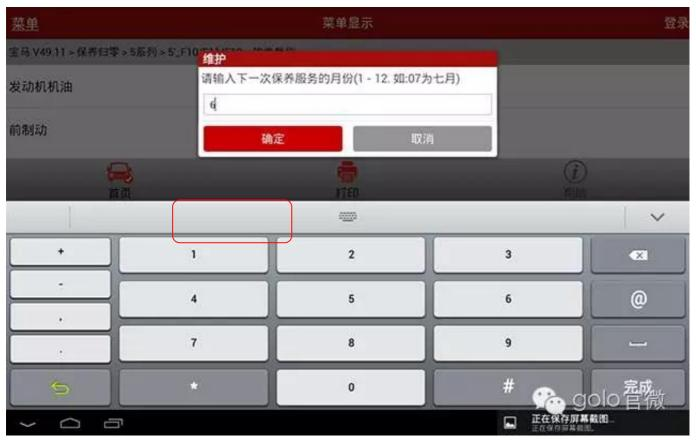
3.2. Vehicle inspection date adjustment, according to the prompts for a month, and year information, the following to adjust to June 2018, for example
