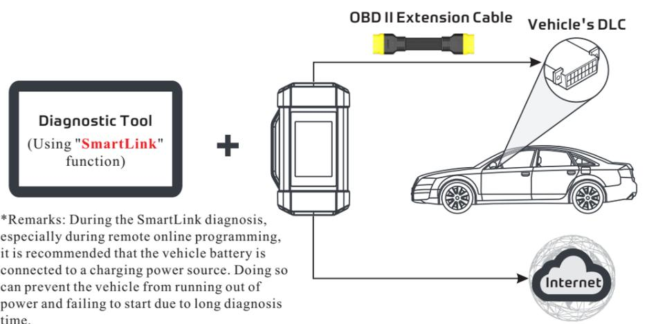
**\*Remarks:** During the SmartLink diagnosis, especially during remote online programming, it is recommended that the vehicle battery is connected to a charging power source. Doing so can prevent the vehicle from running out of power and failing to start due to long diagnosis time.
