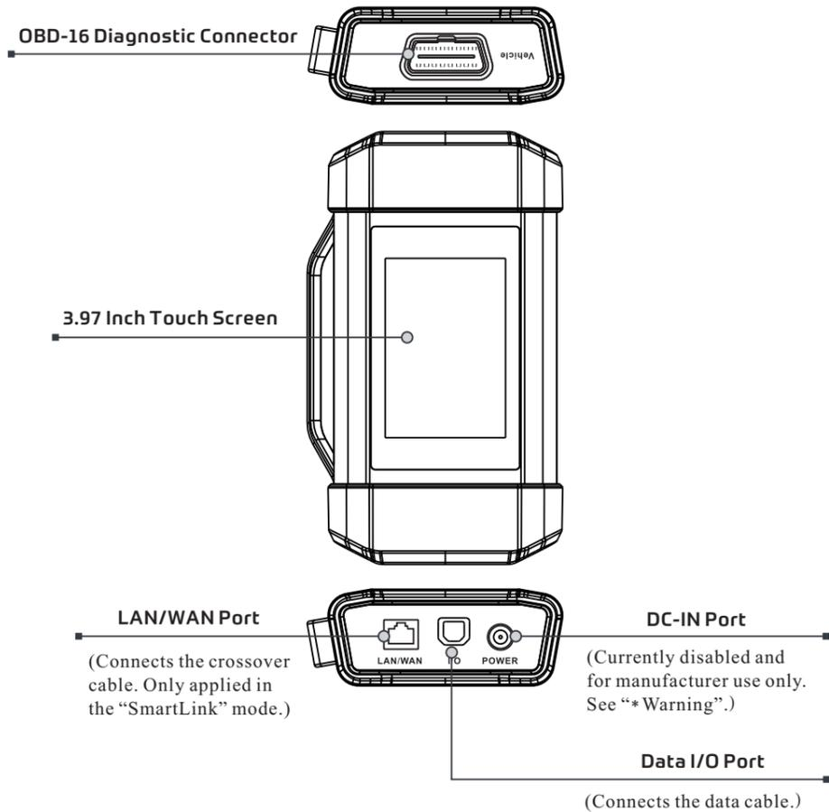
**\*Warning:** The SmartLink C dongle obtains power through the vehicle's DLC, and it is prohibited to connect to an external DC power supply. No responsibility can be assumed for any damage or loss caused as a result of not strictly following the above method.
