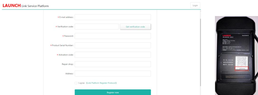
Input your email address and click "Get verification code", platform will send the verification code to your email box. "Product Serial Number" and "Activation code" are pasted as "S/N" and "A/C" on the rear side of Smartlink C device.
