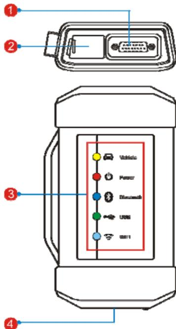
1 Diagnostic socket: For connecting the diagnostic cable.
