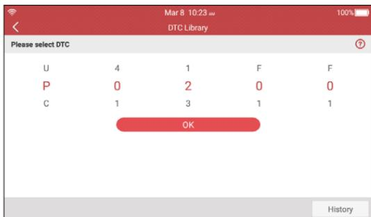
Swipe the screen upwards/downwards to alter the value, then press [OK] button, the screen will display definition of the DTC.
