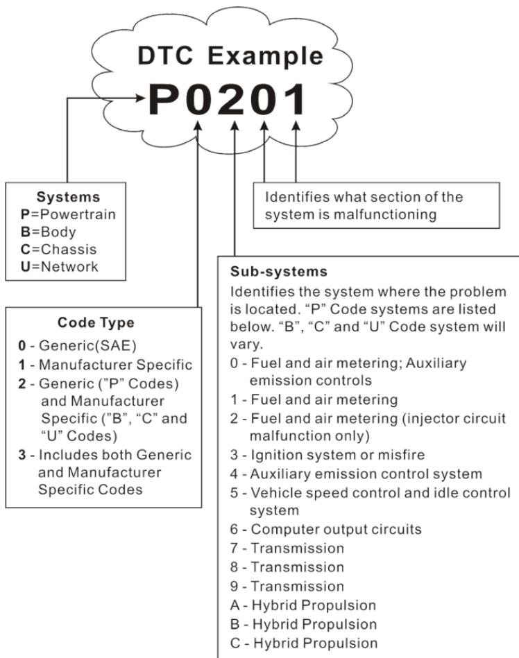
P0201 - Injector circuit malfunction, Cylinder 1
