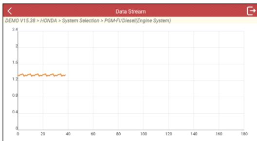
**Combine:** Tap it, a pull-down list of the data stream items appears on the screen. Select the necessary items and the screen will display the waveforms corresponding to these items immediately.
