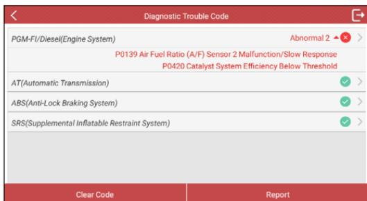
In above figure, the tested system with fault code appears in red and the system with OK displays in black (normally).
